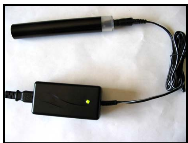
LED on charger module indicates charge condition
